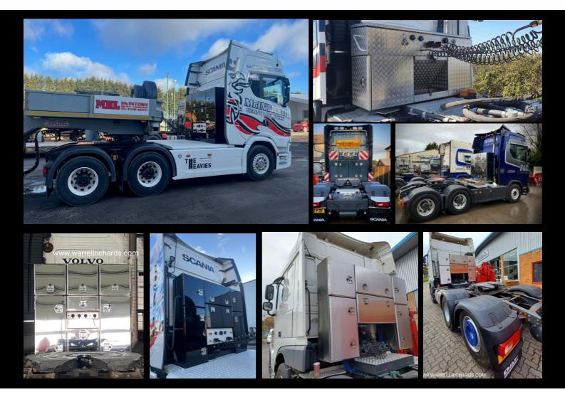
1.5mm Polished stainless finish body with superbright mirrored stainless door, 304 Grade This material is not to be mistaken for the bright annealed mirror finish,
