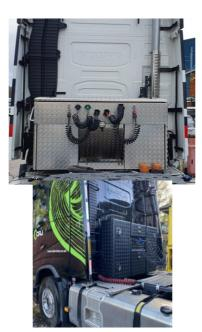
Aluminium chequerplate - 2mm at base / 3.5mm to bars
